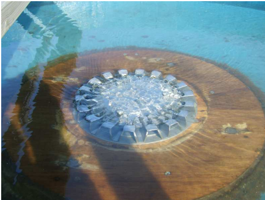
Photograph 1 – Outlet under test at 55mm water depth
